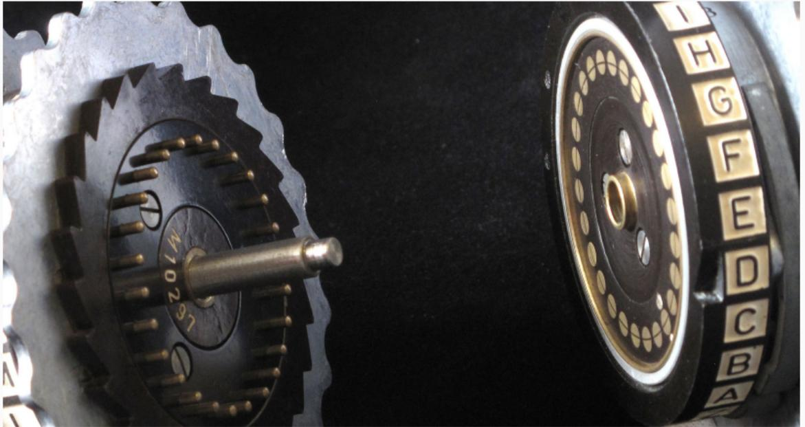
Note the electrical contacts and the ratcheted stepping mechanism.
